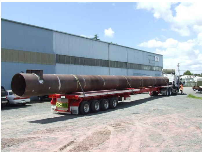
Penstock Piping ready for transport to the painters with Workshop in the background
