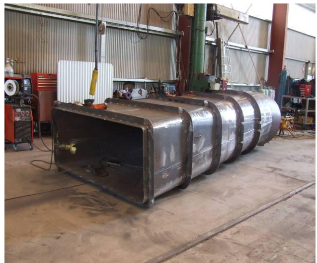
Outfall Transition – Rectangular to round transition.
